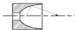
Elliptical Set Screw Reflectors Material Aluminum - Machined and Polished**
